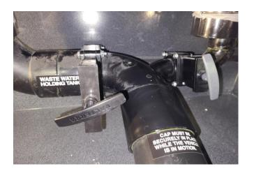
Step 2: Locate your low point drains and open your valves to drain water out of the system close after no more water comes out
