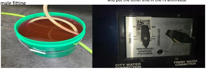
Step 9: go inside the coach and turn on the water pump the pump will begin to pump rv antifreeze into the system the pump will shut off when the system is pressurized
