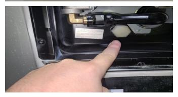
Step:5 remove the water filter cap. Take out the element, dump out water and reinstall the cap
